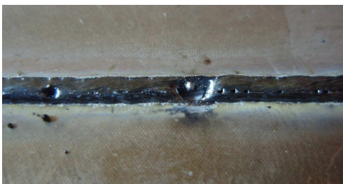
Figure 8 Top-view of case 6, Zn-coated with holes
