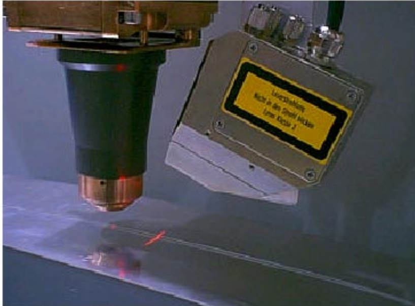
Picture 3: Seam tracking the camera is guiding a welding head for Nd:YAG laser Welding
