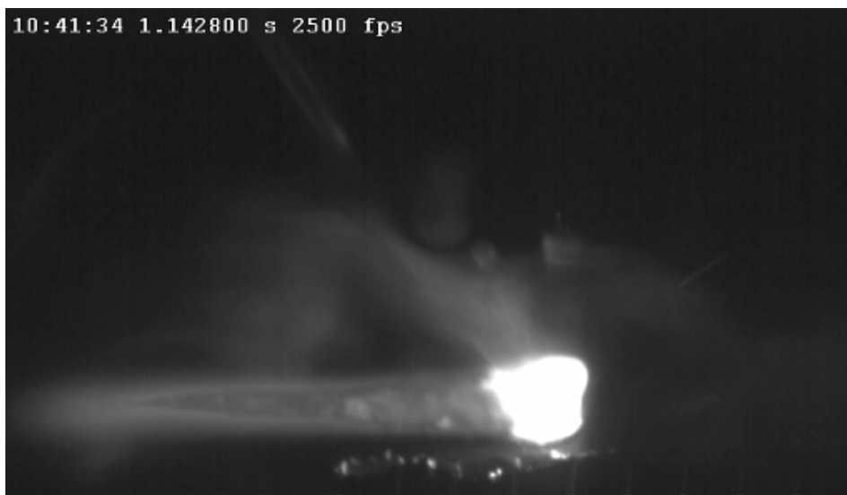
Fig. 15 Frame during weld in zinc coated overlap weld with long melt pool.
