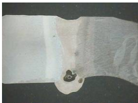
Fig. 9 (a): Cross section with undercut and root sagging
