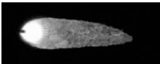
Fig. 2.8.6. Camera-recorded image of the weld-pool area for a non-ideal butt weld configuration: The missing white area in the front part of the keyhole areal is due to a gap between the parts to be welded.
